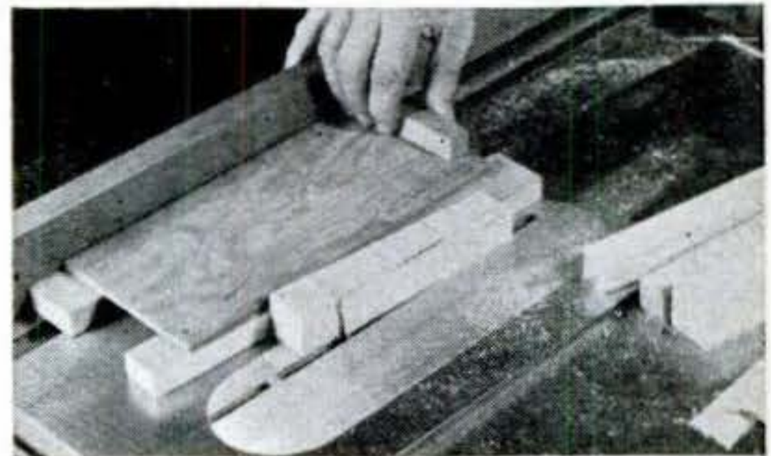
THE JIG IS GUIDED by the rip fence. Fingers need not come near blade. Little finger straddles fence.
